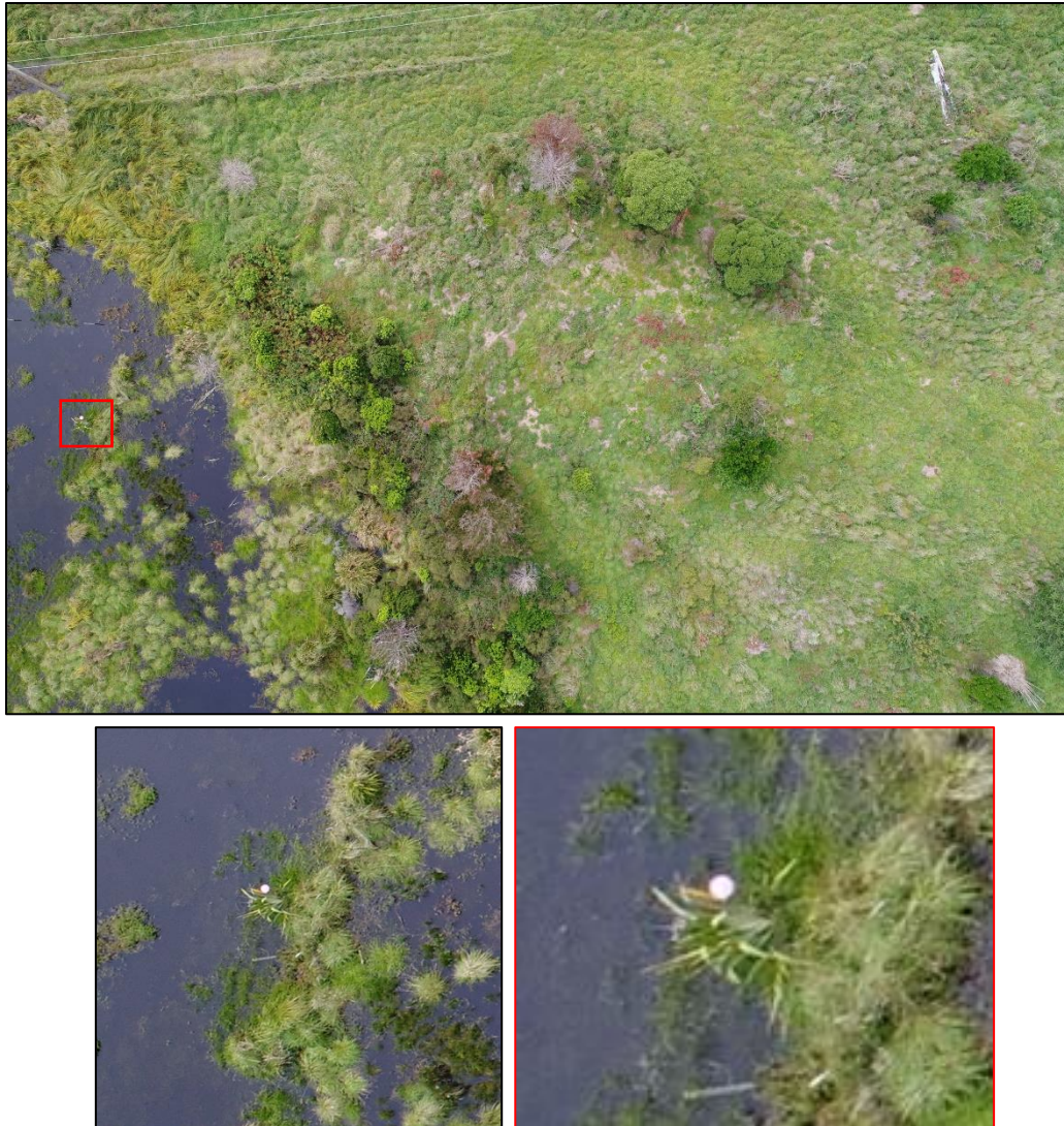
Figure 4. Example of balloon used as a GCP. One of the confines with obtaining accurate and repeatable survey options among aquatic areas is the need for GCPs. Pink party balloons were used to meet the constraints of using GCPs in an aquatic environment. One downside to this method was the time it took to place each balloon, measure the GPS location, and fly the sUAS without the balloon popping. If this area were in need of continued monitoring, then placing a series of permanent poles having visible markings from a nadir perspective would be beneficial. This way, assessment time in the field would only be as long as the flight plan, and permanent GCPs allow for a consistent baseline for temporal comparisons.
